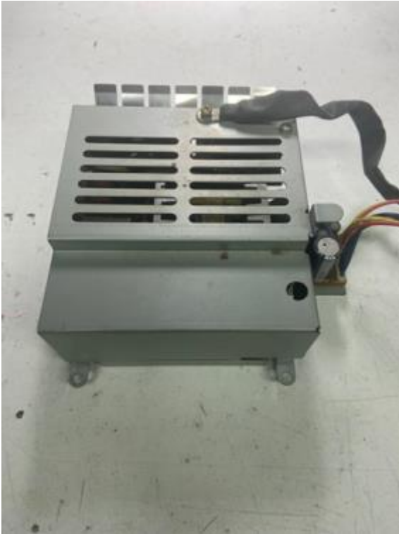
The power supply of the VG 8235/00.
